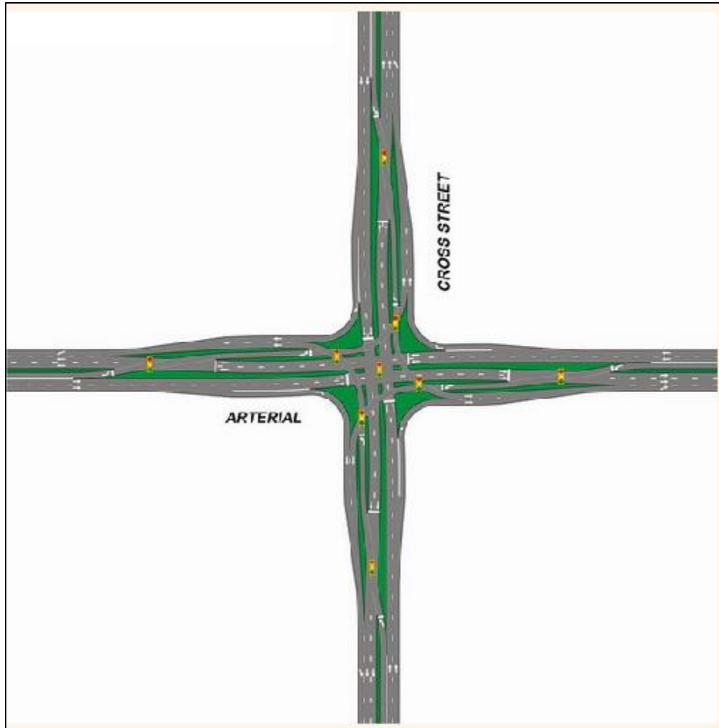
Figure 17: Concept Design of CFI Intersection Geometric Improvement
